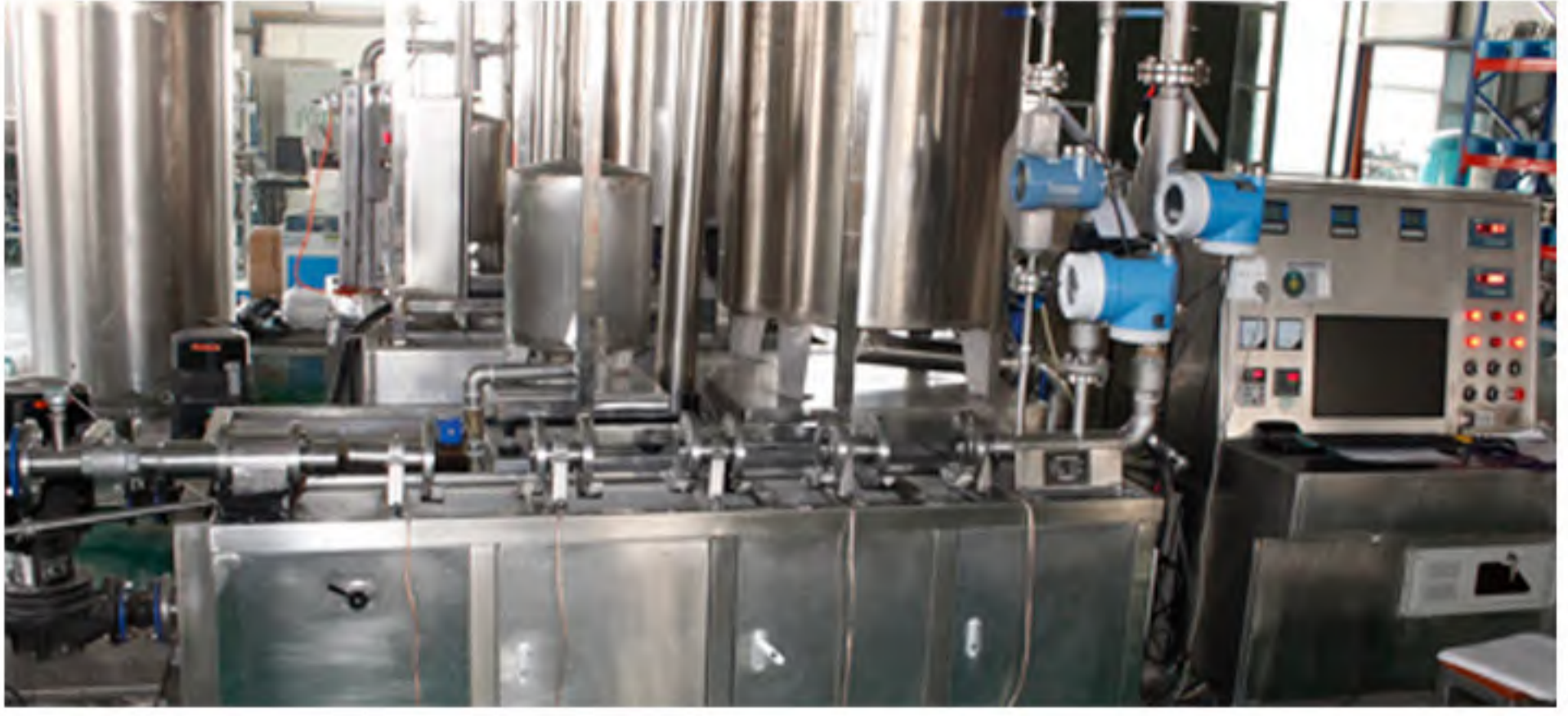
DN15-50 Gravimetric & Standard Meter Liquid Flow Meter Calibration Device
